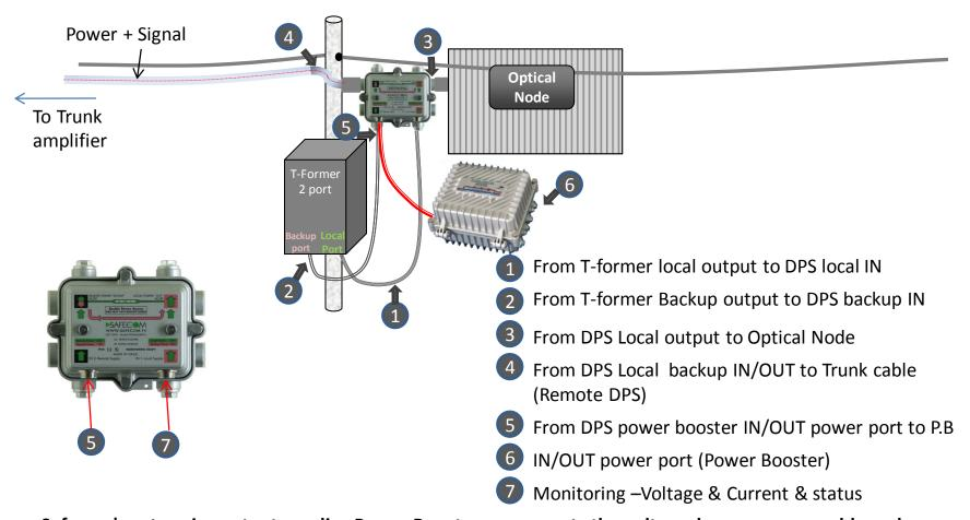
Safecom' cost-saving patent pending Power Booster compensate the voltage drop over coax cable and enables to utilize the DPS technology between remote locations. The Power Booster can be seamlessly connected via cable to the DPS4 enabling robust power redundancy system and overcome the range limitation of the previous DPS
